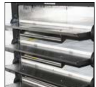
Adjustable Dampers at each deck
