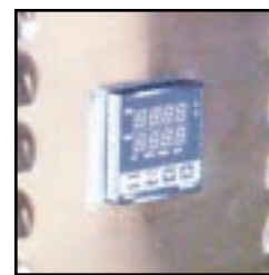
Digital Electronic Controller
